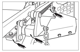
Figure 21. Deck Lift Linkage Pivots
